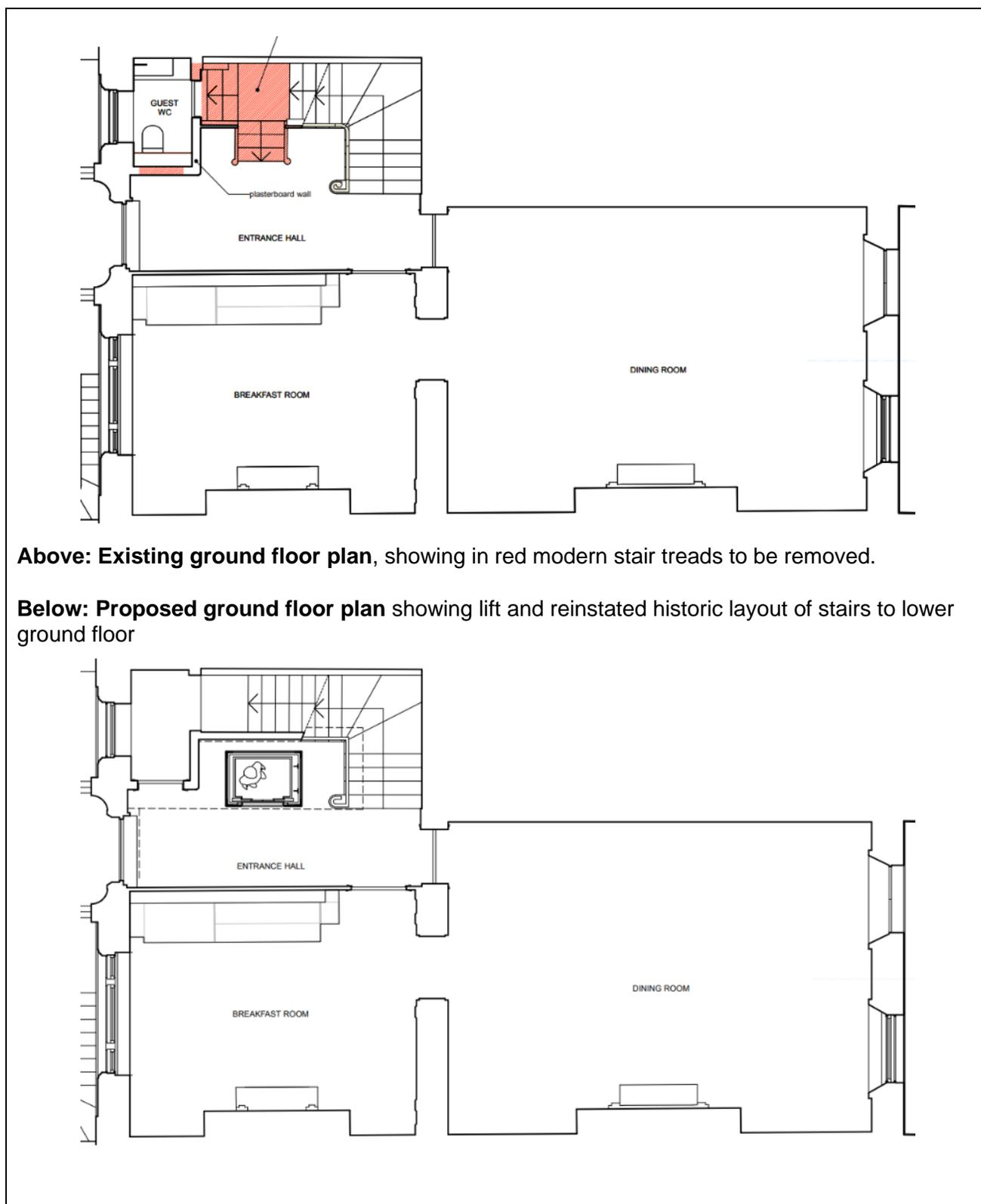
**Above: Existing ground floor plan**, showing in red modern stair treads to be removed.
