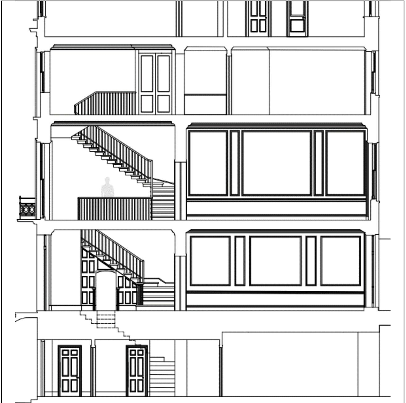
**Existing section** through building, showing open stairwell, and existing modern arrangements at ground to lower ground, and at second floor.
